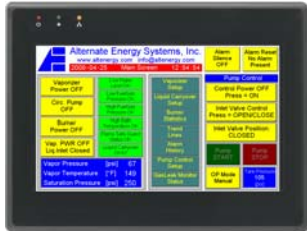
Standard EOI for Siemens PLC S7-1200 or S7-200, optional for Allen-Bradley PLC MicroLogix-1100: 7-inch high-resolution (800x480) display with first-out monitor (Alarm History) and 30-hour graphic TrendLine recording.
