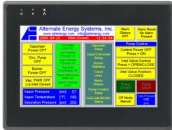
Standard EOI for Siemens S7-1200, Siemens S7-200, or Allen-Bradley MicroLogix-1100: 7-inch high-resolution (800x480) display with first-out monitor (Alarm History) 96-hour graphic TrendLine recording, trend data recording on standard SD card and remote access for monitoring and control via VNC Server / Ethernet. (unlimited client software license included).
